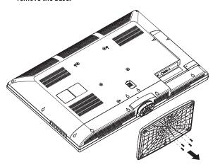
3 Remove the four screws that secure the stand column, then remove the column.
